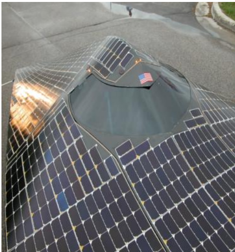
Below left: Principia's Car Ra 7 uses gallium arsenide (GaAs) cells. (photo credits: Terry Zdan)
